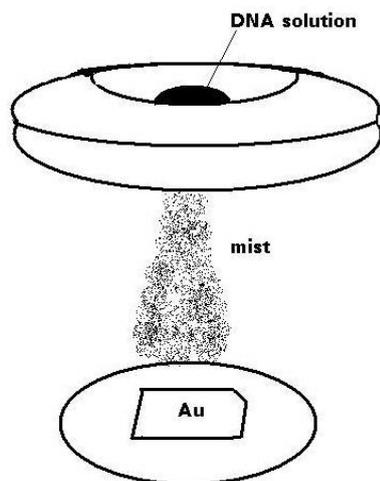
Fig. 1: The schematic diagram of a doughnut shape ultrasonic humidifier. A drop of DNA solution was deposited onto an ultrasonic humidifier. Solution drop became a stream of mist for 3 to 7 seconds usually. Annealed gold strip on a mount was exposed to the mist at a distance of 15 cm away from the humidifier.
