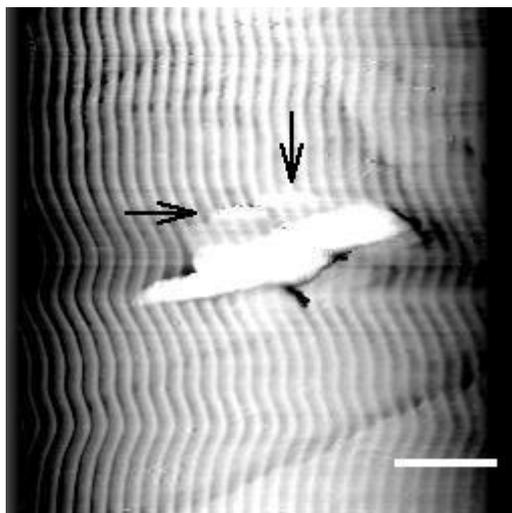
Fig. 3: The image was taken by STM in air, and its size is  $0.5 \mu\text{m} \times 0.5 \mu\text{m}$ . The scale bar represents 100 nm. Exposing annealed gold strip to a stream of DNA contained mist, two individual supercoiled plasmid pUC19 molecules (pointed by arrows) were close to aggregation of other pUC19 supercoiled DNA molecules.
