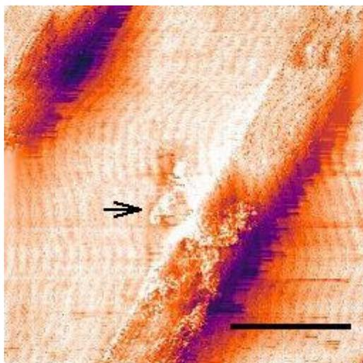
Fig. 2: The image was taken by STM in air and its size is  $1.5 \mu\text{m} \times 1.5 \mu\text{m}$ . The scale bar represents 500 nm. The annealed gold surface formed as terraces. An individual DNA molecule of bacteriophage  $\Phi$ X174 was observed on gold surface near the edge of terrace as indicated by an arrow.
