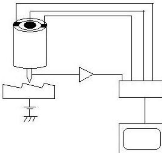
Fig. 1: The schematic diagram of the ambient scanning tunneling microscope.
