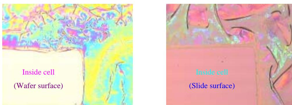
**Figure 2.** Polyimide layer has been completely etched. Left: A silicon wafer piece was used as substrate. Right: Glass slide was used as substrate. Magnifications are same as in *Fig. 1*.
