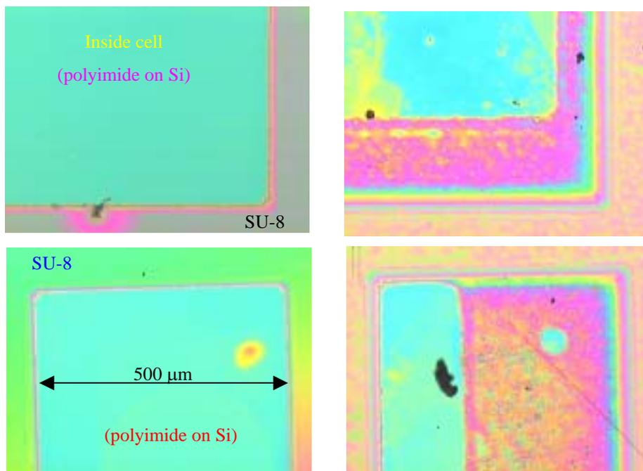
Figure 1. Differences are seen between 5-sec (left row) and 10-sec (right row) exposures. [Images, with same magnification, were taken after developing.]
